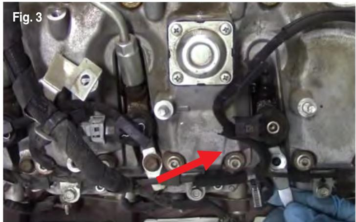
6. Remove the injector bracket bolts and use either GM Tool PN: J-46594 to break the injector free, or a flat head screwdriver to get in between the hold down bracket and seat. If using the flat head screwdriver, gently rock up and down until you feel the injector break free. Any aggressive force can cause damage to other components and or damage the valuable core of the old injector. Once free, the injector can be pulled out by hand (Fig. 3).
