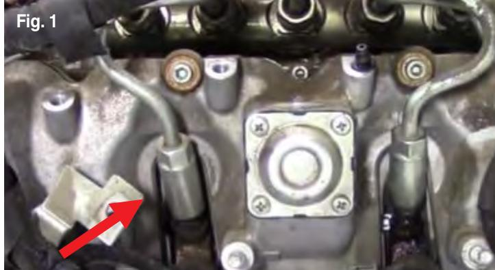
3. Use compressed shop air to blow any debris or contaminants away from the fuel feed tubes to ensure no debris has broken loose or fallen into the injector bore during injector removal. Spray or apply some lithium grease around the tube ends to catch potential debris as the tubes are being removed (Fig. 1).
