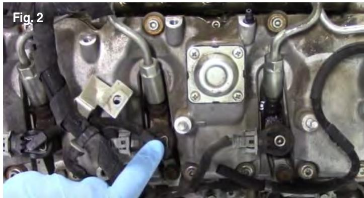
4. Disconnect the fuel return line from the injectors. Be careful not to apply too much force or wiggle the T-connector side-to-side. Simply remove the clip and pull straight up on the T-connector. There should be very little resistance when removing (Fig. 2).
