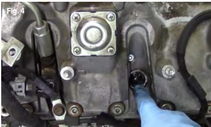
8. Inspect the injector bore for debris and follow the next steps to ensure that the bore is clean and prepared for the new injector (Fig. 4).
