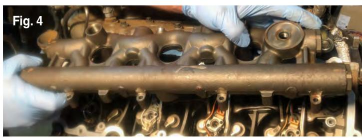
2. Remove the standpipe, dummy plug and manifold bolts, followed by the high pressure oil manifold (Figs. 2-4).
