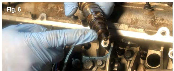
4. Inspect the injector and make sure that the copper O-ring around the nozzle came out along with the injector that is being replaced (Fig. 6).
