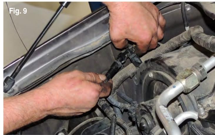
**11.** Prior to starting the engine, it is critical that oil pressure is built and reaches the new injector prior to them operating for the first time. Failure to do so can result in immediate and premature failure of the new injector. To build the oil pressure, locate the wire wrapped in a black sheath running along the passenger side fender that leads to quick disconnect (Fig. 9).
