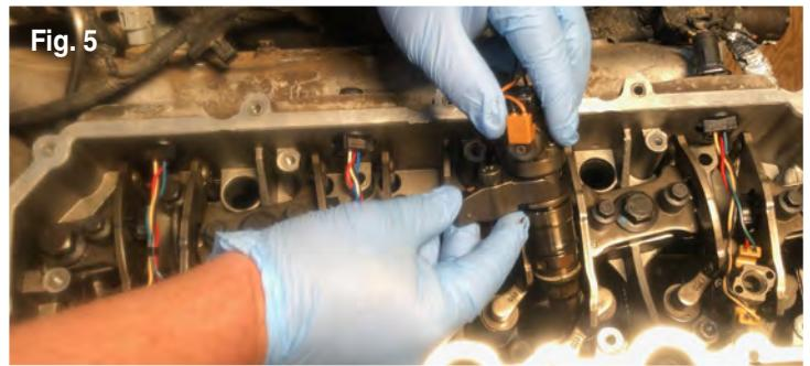
3. Once the injectors are visible, use a LONG SHANK T45 TORX Bit to remove the injector hold down bolt from the injector hold down collar (Fig. 5). Then remove the injector and collar at the same time. If replacing more than one injector, keep the collar and bolt separate and reuse in the same cylinder.
