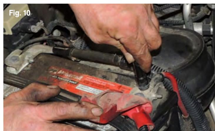
**12.** Disconnect and take the wire over to the positive terminal of the battery. Place the end of the wire on the terminal and allow the engine to turn over for 20-30 seconds (Fig. 10). Repeat this step 3-4 times and then reconnect the wire. You are now ready to start the engine.
