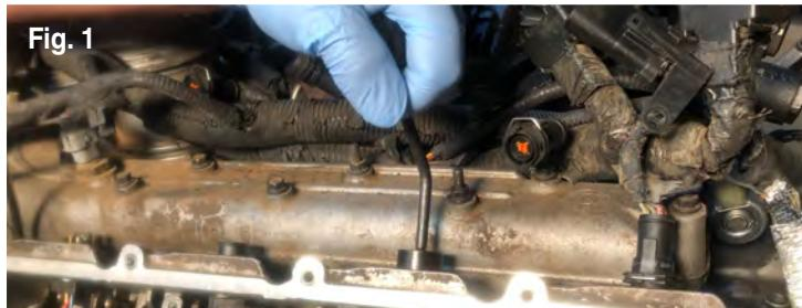
1. Disconnect the fuel injector electrical connector using the special release tool (Fig. 1).
