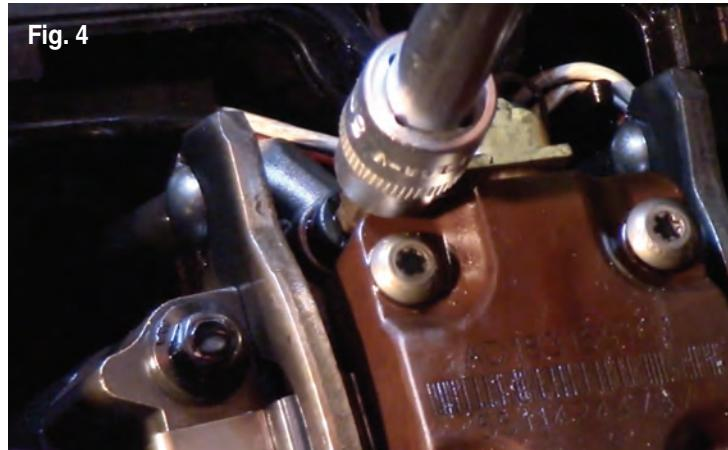
3. Remove the bolt and the oil deflector from the fuel injector hold-down plate. If replacing more than one injector, be sure to keep each bolt and deflector with the original cylinder from which they were removed (Fig. 4).
