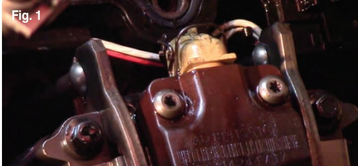
1. Disconnect the electrical harness found on the valve cover gasket from each injector (Fig. 1). For easier removal and installation, disconnection and removal of the entire gasket is recommended while following the next steps.
