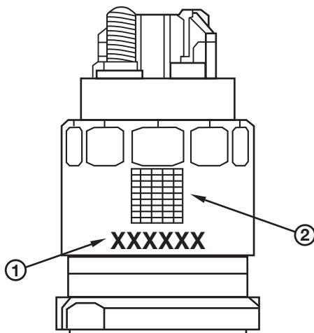
6. Each new fuel injector has a six-digit alphanumeric correction code. The correction code is printed on the intake side of the fuel injector and is used to identify injector calibration. When replacing any fuel injectors,
