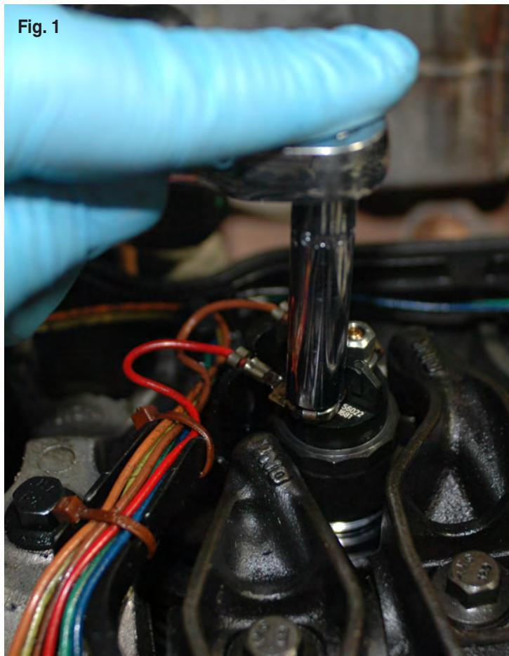
2. Remove the electrical connector nuts from the injector and move the harness away from the injector. The nuts should be a part of the wiring harness. If they come off, use caution to not drop it into the engine and do not reuse. Install a new valve cover gasket assembly (Fig.1).
