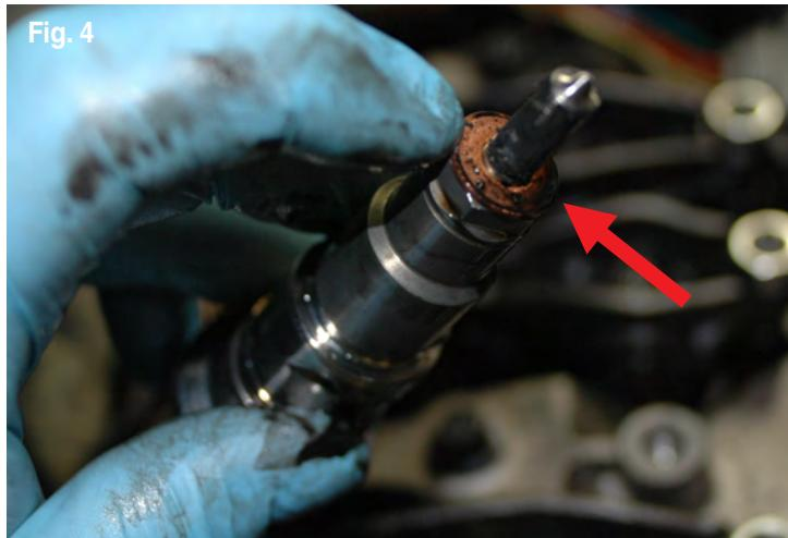
5. After the injector is free, visually verify that the copper washer around the nozzle came out as well. If not, check the bore and remove the washer. Failure to do so can and will result in the replacement injector not torquing properly and leak (Fig. 4).
