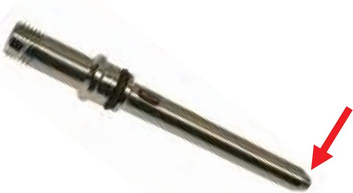
10. As mentioned in the beginning of this guide, it is recommended that the connector tubes be replaced. If reusing, inspect the taper of the connector. If visible grooves or scarring are found, the ability of the connector to create a seal is unlikely and there will be a leak (Fig. 6).
