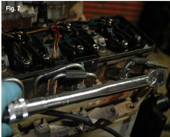
12. Do a final tightening of the Feed / Connector Tube and retaining nut. Tighten to **50N.m (37 ft-lbs torque)**. (Fig. 7).
