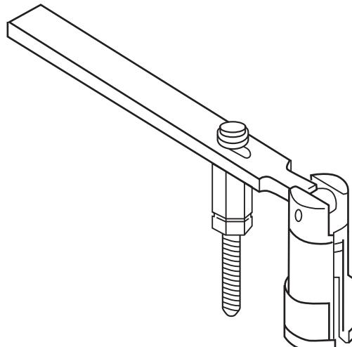
4. With the connectors, exhaust rocker arm and feed tubes removed, you can now pull up on the injector and remove it from the bore. If you find that the injector is seized or difficult to remove, use the recommended specialty tool #9010 to clamp around the injector for removal. Use of other tools can damage the injector (Fig. 3).
