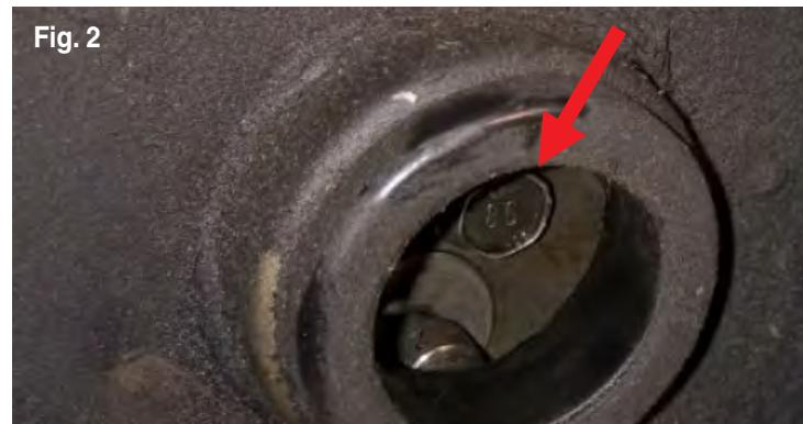
1. Removing the oil fill tube gives you access to the pump retaining bolts. An important tip is to remove the grommet that seals the fill tube to the timing cover. The opening is very tight with the grommet in place. Injection pump removal labor will double if the retaining bolts are dropped into the timing cover. See images and red arrows for reference. (Fig. 1 and Fig. 2).
