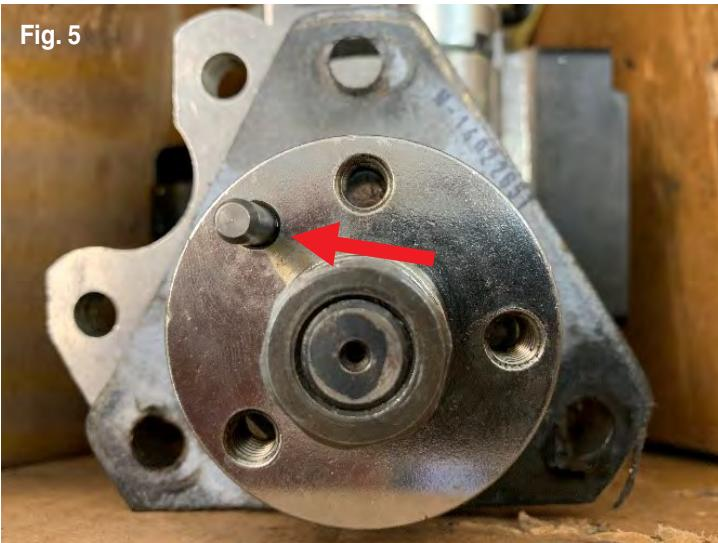
10. Install the fuel injection pump gear. Make sure to align the slot in the injection pump gear with the location pin on the fuel injection pump hub. (Fig. 5).
