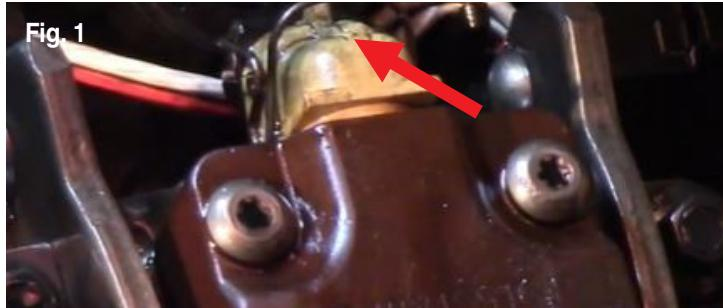
1. Disconnect the electrical harness found on the valve cover gasket from each injector. For easier removal and installation, disconnect and remove the entire gasket. (Fig. 1).
