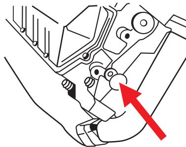
12. Replace and tighten the cylinder head drain plugs from the second step in this process and replace the valve cover gasket and cover. To ensure proper lubrication and supply at start up, prime the fuel to the injectors by turning the key to ACC for 15 seconds and then off. Repeat 3-4 times, then start the vehicle (Fig. 10).
