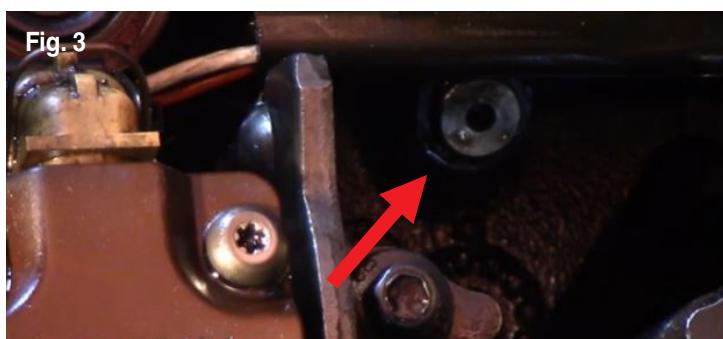
3. Loosen the drain plugs located at the rear of each cylinder head. Doing so will assist in the drain back of fluids that should not enter the combustion chamber (Fig. 3).
