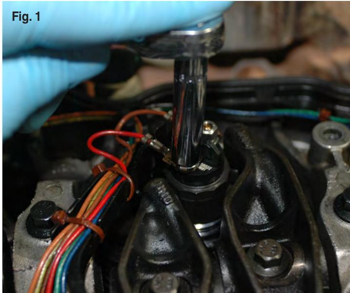
2. Remove the electrical connector nuts to the injector and lay to the side. Each electrical connector nut should remain attached to its wiring harness connector end. If any connector nut does not remain attached, care should be taken to ensure that it does not fall into vulnerable areas of the engine. If replacing all six injectors, it is easiest to disconnect all connectors and remove the valve cover gasket completely (Fig. 1).
