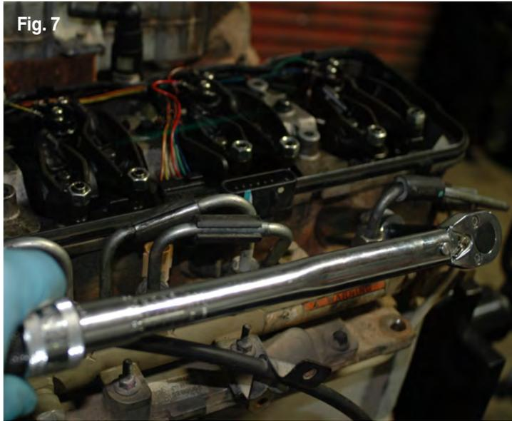
12. Do a final tightening of the new Feed / Connector tube and retaining nut.
