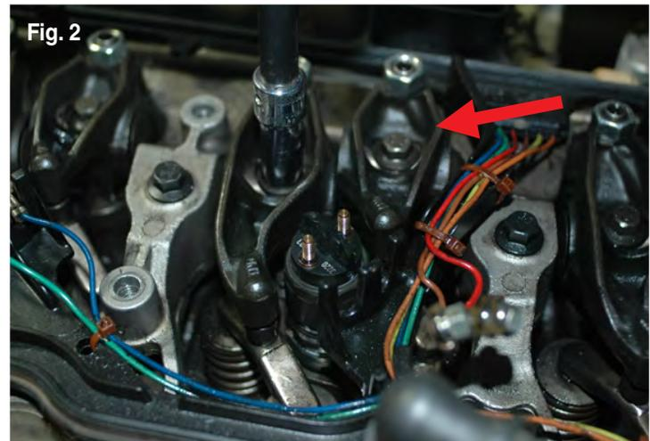
3. Remove the Exhaust Rocker Arm Assemblies corresponding to the injectors being replaced. Mark and / or organize these to ensure they make their way back to the cylinder they originally came from (Fig. 2).
