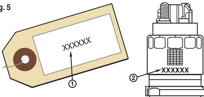
7. Each new fuel injector has a six-digit alphanumeric correction code used to identify injector calibration. When replacing any fuel injector, this code must be entered into the vehicle's Engine Control Module (ECM) using a diagnostic scan tool. Do not install new fuel injectors unless the alphanumeric codes have been recorded. The correction code is printed on a tag that is attached to the injector (1). If there is no tag present, please use the correction code
