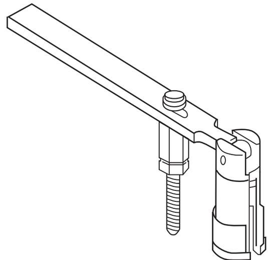
4. With the connectors, exhaust rocker arm and feed tubes removed, you can now pull up on the injector and remove it from the bore. If you find that the injector is seized or difficult to remove, use the recommended Specialty tool #9010 in (Fig. 3) to clamp around the injector for removal. Use of other tools can damage the injector.
